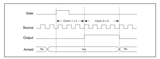
**Figure 2-20.** Single Triggered Pulse Generation
